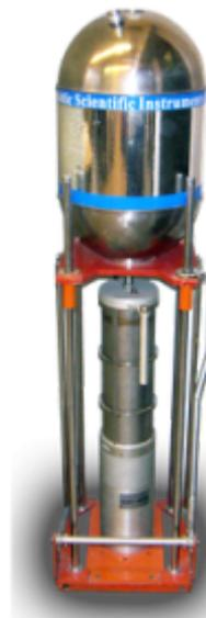
Deep-Water gamma-spectrometer is applicable to the registration of gamma-radiation from radionuclides in monitoring of the sea bed for objects from marine accidents, submarine storage of radioactive wastes, search of lost nuclear charges, inspection of radionuclide migration, etc.
