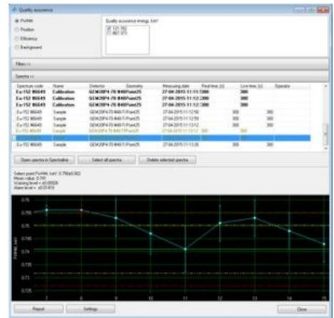
The reference sample and the background are measured in semi-automatic mode for quality control. As the scenarios are used the measurement parameters can be flexibly adjusted and the monitoring results can be displayed depending on the date and time of the measurement start.
