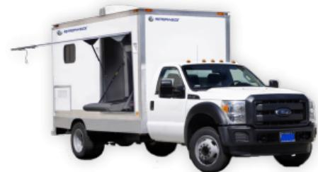
The X-ray system is custom built into a Ford F-450 Super Duty Truck complete with cabin air conditioning, a 6.2L V8 engine and the Ford Personal Safety System.
