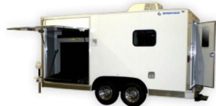
Significantly, this mobile screening vehicle is the first in its class in terms of standard equipment. The XIS Trailer is equipped with a powerful 180 kV generator, air conditioning, exterior lighting and uninterrupted power supply.
