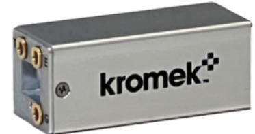
The Kromek GR family is a range of CZT-based high-performance Gamma spectrometers. They are completely self-contained, with built-in preamplifier, shaping amplifier, baseline restorer, pulse height digitizer and HV supply. The digitised pulse heights of detected Gamma signals are sent to a computer via the USB. The unit is powered entirely from the USB bus, so no external power supply is needed.
