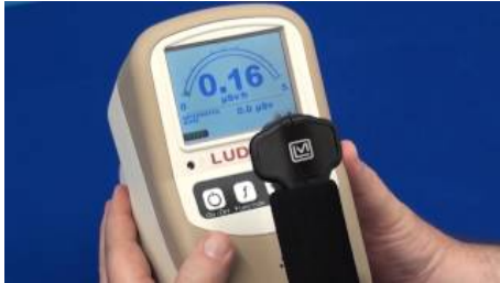
9DP control panel overview
