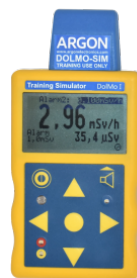
Nuvia DoMo Radiation Hazard Detection Simulator
