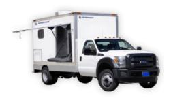
The X-ray system is custom built into a Ford F-450 Super Duty Truck complete with cabin air conditioning, a 6.2L V8 engine and the Ford Personal Safety System.
