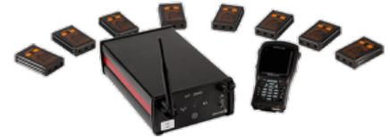
The operational dosimetry system Skydose consists in eight Saphydose  $\gamma$  RT teledosimeters, one Personal Digital Assistant (PDA), one Easydose configuration software, one Saphyr portable reader, as well as one to three RT-ZB05 routers.
