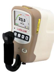
**Model 9DP-1 Pressurized Ion Chamber**
