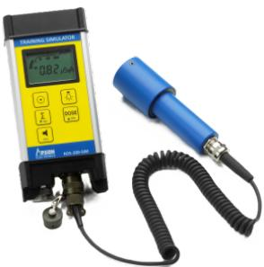
**M4A1 JCAD Chemical Hazard Detection Simulator**
