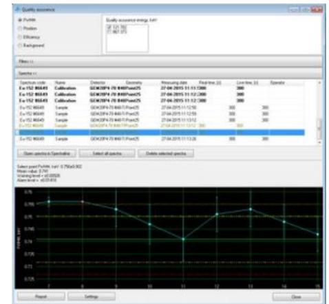
The reference sample and the background are measured in semi-automatic mode for quality control. As the scenarios are used the measurement parameters can be flexibly adjusted and the monitoring results can be displayed depending on the date and time of the measurement start.
