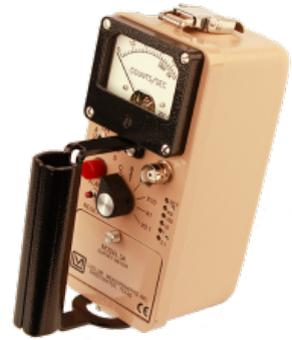
The front-panel controls include a rotary switch for selecting the four-decade range, instrument shut-off, and battery test, an audio on/off switch, a fast/slow response switch, and a count reset button. The analog meter comes in a variety of measurement ranges and units to support the external radiation detector selected.
