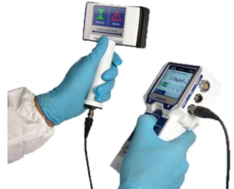
SaphyRAD's wide range of contamination probes combined with its specific algorithm allow for a very fast and reactive detection. Depending on the probe, the operator can either assess small or large areas to detect alpha, beta/gamma or alpha & beta/gamma radioactive contamination. All data can be stored on an SD card for measurement recordings.
