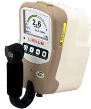
Measurements and instrument status are displayed on a large 232K-color, backlit LCD screen. The screen displays the current exposure rate as well as simultaneously displaying either the integrated exposure rate or the peak exposure rate in Sv, R, Gy, or rem units. An additional mode, Pulsed Mode, locks the instrument in the highest measurement range in order to improve pulsed radiation response while sacrificing low radiation reading resolution.
