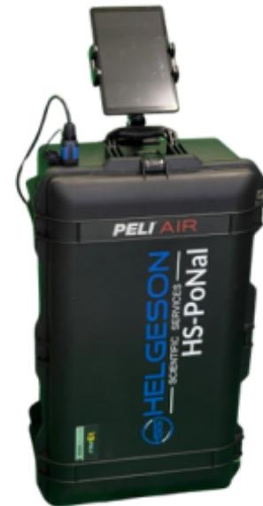
HS-PoNaI is a fantastic solution for a quick and efficient **in-situ isotope identification** in different applications. It is a strong and customizable equipment with a very simple and intuitive operation thanks to its automatic isotope identification and quantification software. It is equipped with a 4 liters NaI detector (4x4x16"), and all electronics are installed inside a PeliCase providing IP67 protection. Communication can be done remotely via tablet or another device.
