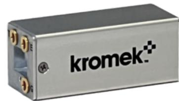
The Kromek GR family is a range of CZT-based high-performance Gamma spectrometers. They are completely self-contained, with built-in preamplifier, shaping amplifier, baseline restorer, pulse height digitizer and HV supply. The digitised pulse heights of detected Gamma signals are sent to a computer via the USB. The unit is powered entirely from the USB bus, so no external power supply is needed.
