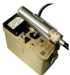
**Model 195 with Model 43-132 High Range Alpha Ion Chamber**
