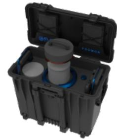
The whole device is self-contained in a portable high-IP-grade technical case, for an overall weight < 25 kg. The food samples are to be placed in 500 ml Marinelli beakers, which then are lodged inside a 1 cm thick lead shielding well upon the detector’s end cap. The complete setup and deployment of the system requires less than 5 minutes.
