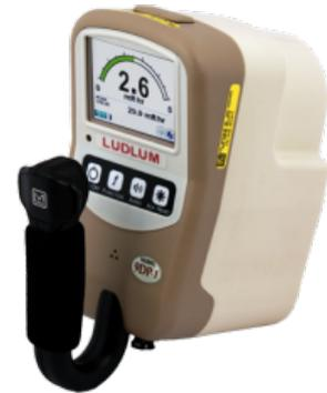
This meter is also specially designed to measure pulsed radiation fields, correctly integrating 50 ns pulses (and wider) that other systems typically miss or measure inaccurately. Another feature is a detector chamber that is only pressurized to 2.5 atm (22 psig), eliminating (USA) shipping and handling HAZMAT concerns. However, this reduced pressure also decreases sensitivity, reducing the minimum measurement point to 2  $\mu\text{Sv/h}$  (200  $\mu\text{R/hr}$ ).
