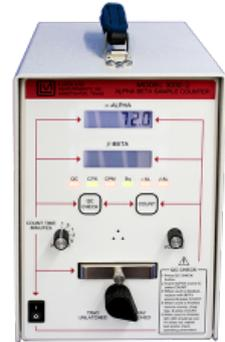
The Model 3030-2 Simultaneous Alpha-Beta Sample Counter is a dual-channel counter designed for simultaneous alpha and beta sample measurement.
