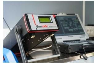
**GammaTRACER Autonomous Radiation Monitoring Probe - Saphymo**
