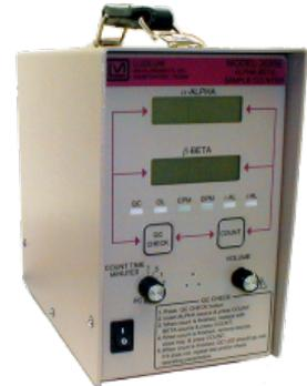
The Model 3030E is a dual channel, scaler-type, sample counter electronics package that will accommodate many detector inputs from external sample head/detectors. This design represents a significant improvement over older analog type scalers by providing greater utility and functionality.
