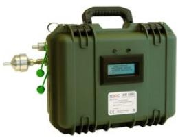
**AM 3000 - Air Sampler for Asbestos Diagnosis - NF43-050 version 2021, NF X43-269, NF EN ISO 13137**
