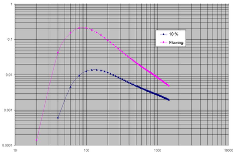
Absolute efficiency registration comparison curves during gamma-ray emission with sample positioning inside and outside detector.
