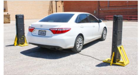
Ease of setup, adjustable audio signals, and user-friendly LCD display that provides detector counts, background levels, and system parameters, and the ability to operate via vehicle cigarette lighter plug or batteries, keep the Model 52-8 applicable to a variety of different situations. This instrument meets the Federal Emergency Management Agency (FEMA) standard for Emergency Management Response Portal Monitoring (FEMA-REP-21).
