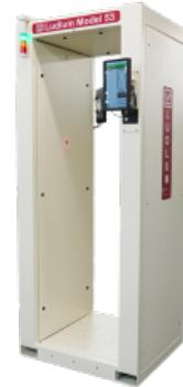
Three statistical counting modes are available to maximize throughput, maximize sensitivity, or fix the count time. Several modifiable parameters adjust the alarm set point, including the false alarm probability, detection probability, background sigma coefficient ( $K_b$ ), and the composite sigma coefficient ( $K_{S+B}$ ). Fast alarm and clean options provide the ability to quickly determine if personnel are contaminated or clean before the entire count cycle has ended.
