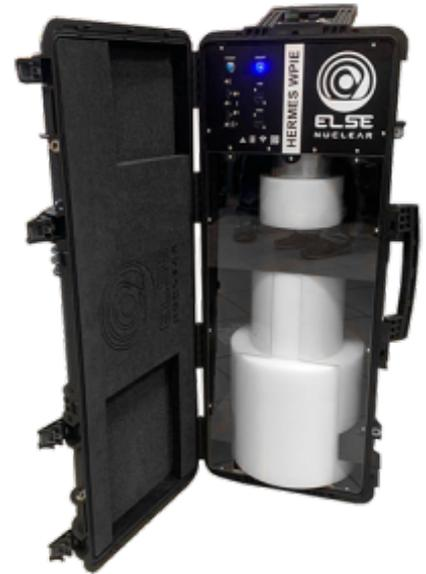
W-PIE employs  $^6\text{Li}$  as neutron converter,  $^4\text{He}$  as scintillating medium, and 24 independent low-voltage SiPMs as photosensitive components. The detector is surrounded by increasingly thick moderating assemblies, defining 4 detection sub-volumes each optimised for a specific spectral region. Signals are acquired and analysed by the built-in electronics and unfolding algorithm, or they can be saved as raw data for off-line analysis.
