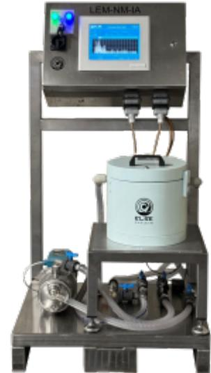
The measurements are visualised in real time by the software, expressed in terms of specific/total activity through spectroscopic analysis.
