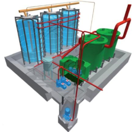
The WDMS NT-VK system is designed to collect and monitor radioactive wastewaters, which can be released only after their radioactivity drops below a defined value. The main application of such a system is related to diagnostic and therapeutic procedures involving radioactive substances, and their partial elimination through the patient's metabolism.
