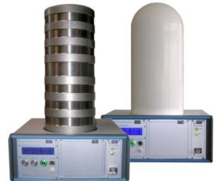
The standard NAUSICAA configuration, suitable for indoor use, is composed by a 3U 63HP table box housing the electronics modules, and the ion chamber directly installed on top of it. Wall mounting accessory and trolley kit are also available, as well as an IP54 enclosure.
