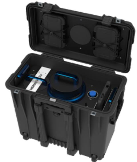
HERMES GSU quantifies isotope activity concentrations based on a rich built-in, yet fully-editable, isotope library. Its portability and autonomous operation make it ideal for both routine monitoring and emergency response scenarios.
