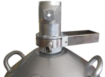
HPGe detector flowing geometry can be developed based on the crystal with equivalent efficiency from 10 to 100%.
