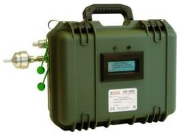
**AM 3000 - Air Sampler for Asbestos Diagnosis - NF43-050 version 2021, NF X43-269, NF EN ISO 13137**
