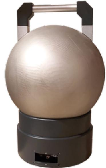
SP2 is characterized by the same high sensitivity and precision as BSS in determining the neutron flux over the entire energy range, while removing any reproducibility uncertainty. When employed with the on-line unfolding tool, SP2 can also perform real time measurements.
