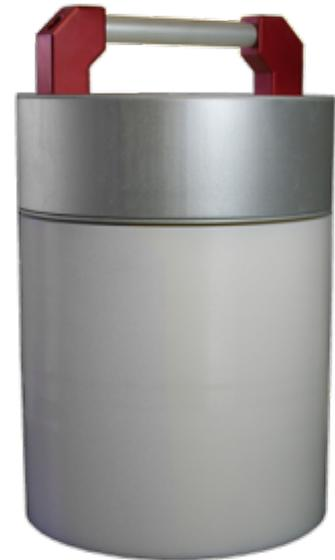
The electronics processes the signal coming from the detector and elaborates the instantaneous  $H^*(10)$  rate value every second.
