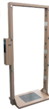
subtract it from the current count. This function helps compensate for fluctuations in background. Background subtract can be turned on or off, the background count time is adjustable, and the background interval time is adjustable. The operator can force the instrument to stop and take a background count at a different interval if desired.
