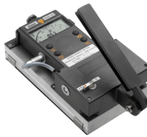
Ludlum 133-6 and 44-2 Radiation Simulation Probes
