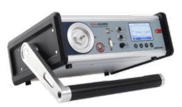
AlphaGUARD incorporates a pulse-counting ionization chamber (alpha spectroscopy).
