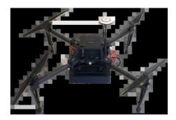
When mounted to any multirotor drone model, Kromek's AARM payload system can be used to complete rapid, detailed radiological surveys over wide areas. Its advanced sensor system of integrated radiation and positional sensors allows isotopic fingerprinting, counts per second, and full spectral data to be collected and subsequently delivered to the user every second.
