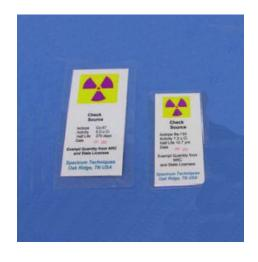
Plastic laminates provide a convenient alternative packaging being easy to handle and store. The standard laminates have a transmission window of 0.005" and produce minimum attenuation for photons and higher energy beta particles.
