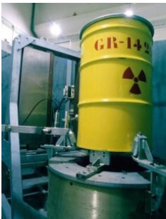
Descaling system for NORM waste
