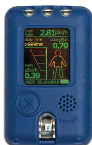
PED-ER (Personal Electronic Dosimeter) - Tracerco
