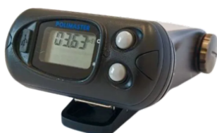
PM1703GNA-II MBT Personal Radiation Detector/Dosimeter
