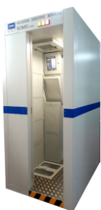
HS-BOMO - Beta gamma portal for personnel monitoring
